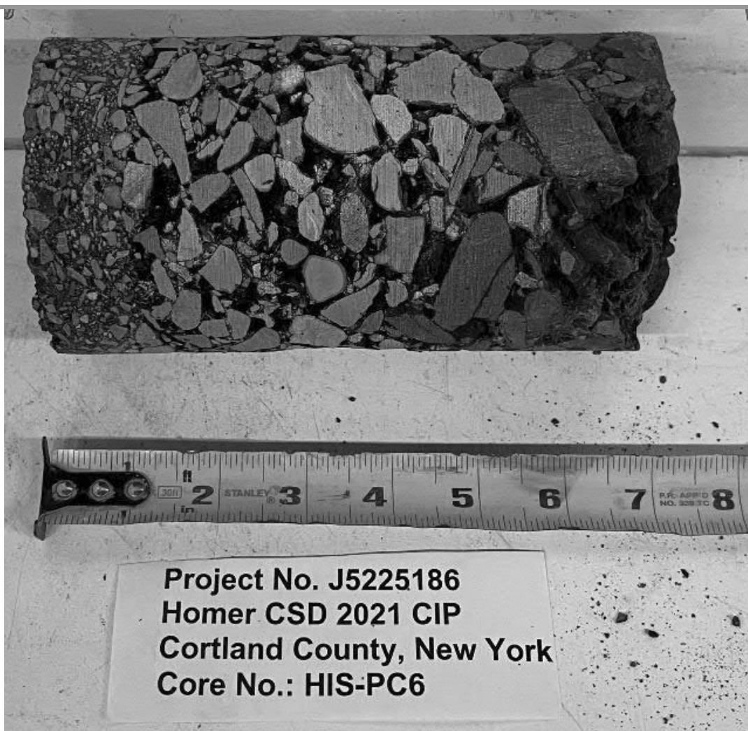
Pavement core at boring HIS-PC6
