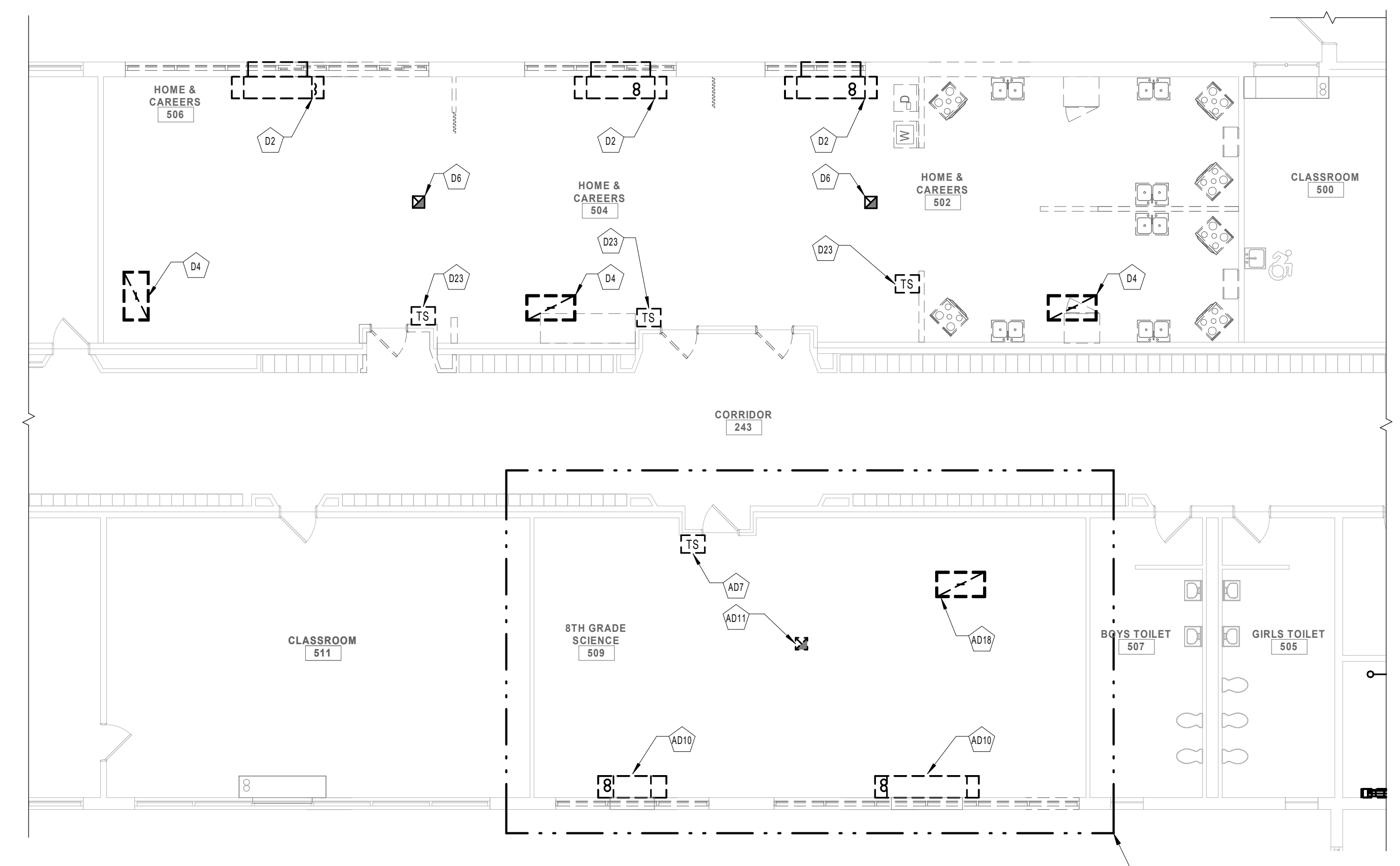
2 FIRST FLOOR DEMOLITION PLAN - AREA D SCALE: 1/8" = 1'-0"
